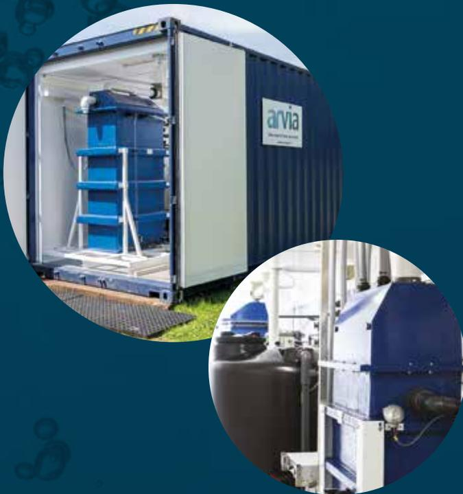
In contrast to traditional advanced oxidation processes (AOPs), results using the Nyex™-a and Nyex™-e processes are achieved without chemical dosing and the production of toxic sludge or secondary waste, which are becoming increasingly expensive for industrial facilities to manage and dispose of.
